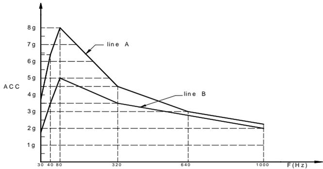
Line A: Maximum acceleration with a 125 gram load vs. frequency.
