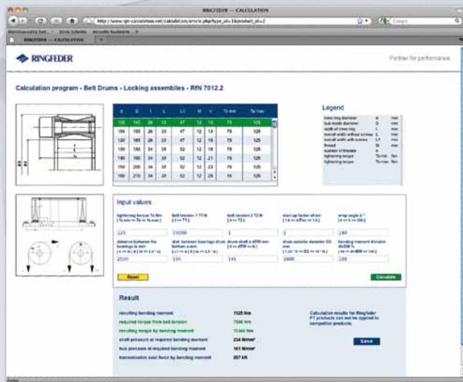
In order to meet the complex requirements on the correct design and selection of RINGFEDER products under bending moment loading, RINGFEDER POWER TRANSMISSION GMBH has developed a calculation program.
